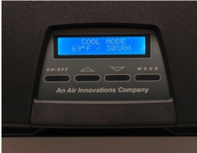
Local interface controller
